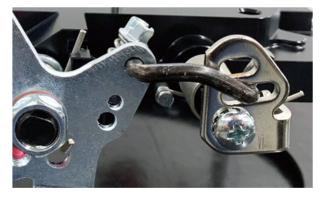
Super Progressive Black Link: top hole, lower slot 60% primary before secondary opens.
