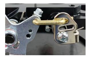
Stock Gold Link: top hole, top slot 40% primary before secondary opens. This is standard for most applications.
